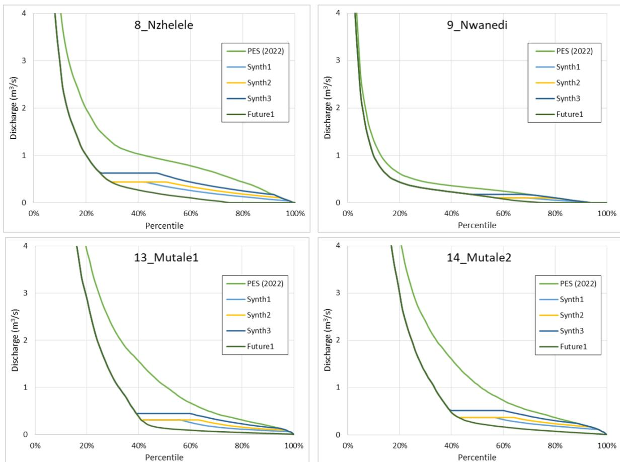
**Figure 7-1** Flow duration curve for PES (2022), Future1 and Synthetic Scenarios 1, 2 and 3
